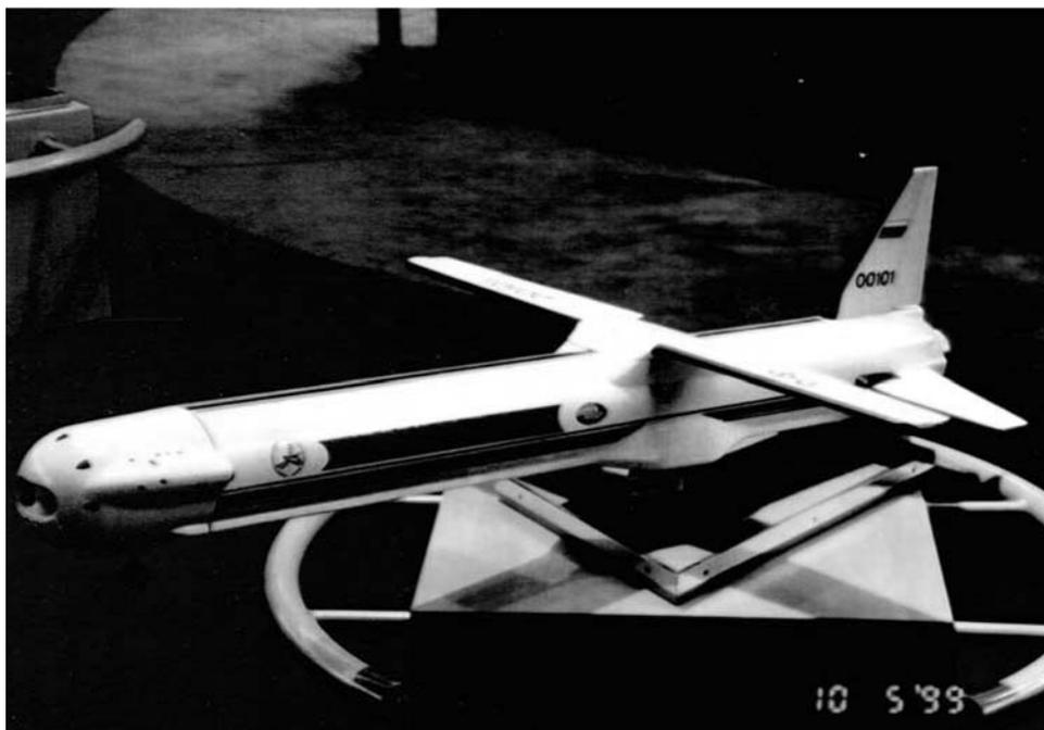
**Figure 2.12.** Fly-back version of the Zenit strap-on as an alternative to lifting parachutes.
