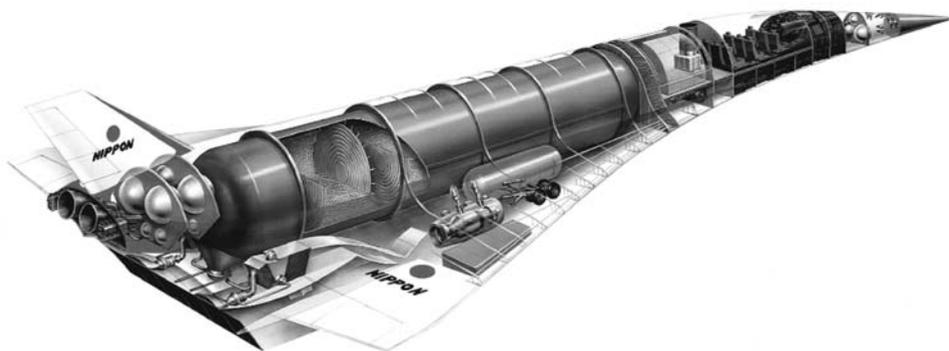
Figure 2.3. Aerospace Plane concept from Japan National Aerospace Laboratories (NAL).
