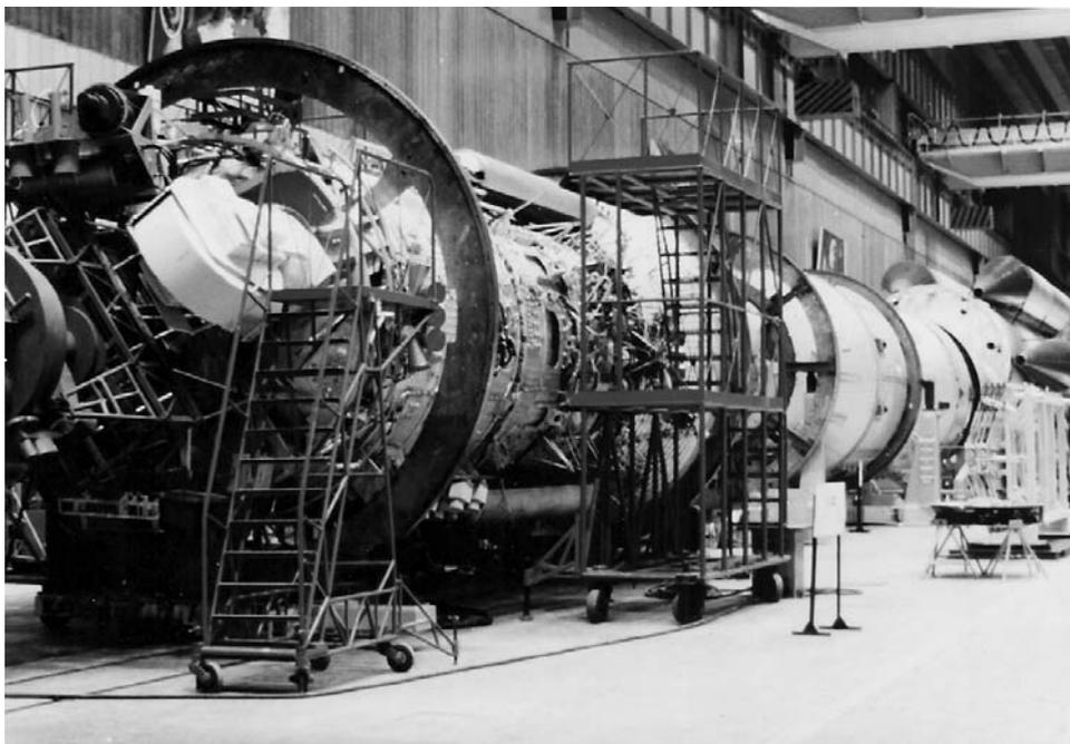
**Figure 5.22.** Large orbital station in final assembly and integration with its Proton booster.
